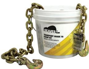
GRADE 70 LASHINGS & FITTINGS ARE NOT TO BE USED FOR LIFTING PURPOSES \* NOTE: The use of some grab hooks or systems incorporating grab hooks cause bending to occur on the link of lashing chain to which the grab hook is engaged. The bending and shearing effect of the hook reduces the strength of the chain by 25 percent and as such, the lashing capacity (LC) of this type of system must be reduced by 25 percent as prescribed in Australian Standard AS/NZS 4344
